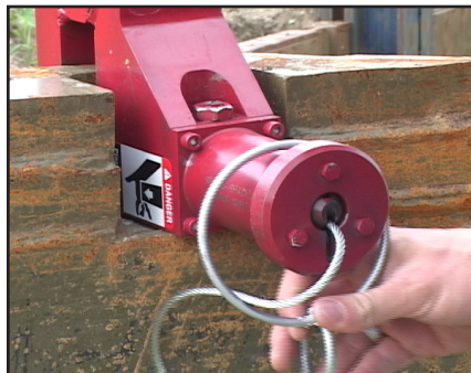
4. Place the safety ring over the housing.
